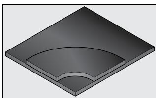
Position both sides together with smooth skin facing out and apply Aerocel adhesive to outer edges.
