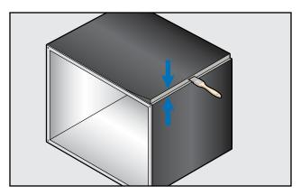
Once adhesive is ready for contact, carefully install glued edge seams flush and with firm pressure under compression to ensure complete contact and vapor seal.
