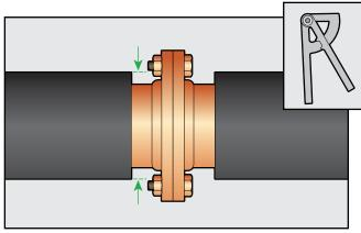
• Using caliper, measure circumference of flange.
