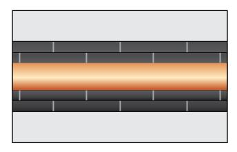
First layer of Aerocel sheets to be installed with full Aerocel adhesive coverage or Aerocel with PSA (pressure-sensitive adhesive back).
