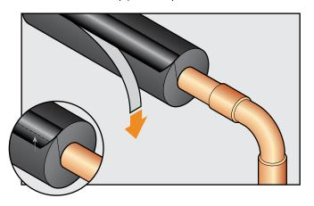
Carefully press Protape double closure seal onto clean outside wall of tube with firm pressure, avoiding any kinks or gaps, until the SSPT tube is fully sealed.
