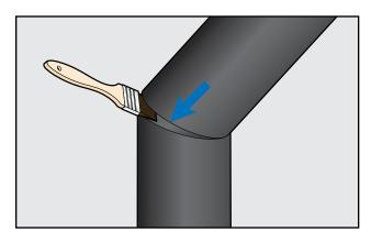
When ready for contact, join longitudinal seam first followed by miter seam with firm pressure under compression.
