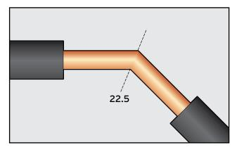
Straight pipe runs are typically insulated up to 45° bend.
