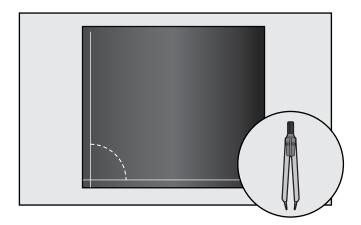
Measure the circumference of pipe using strip of Aerocel Sheet or Roll (same thickness, do not stretch); add 1/4" [.64 cm] to measurement.
