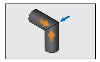
Once 45° seam is bonded, cut inside radius of cover (throat).
