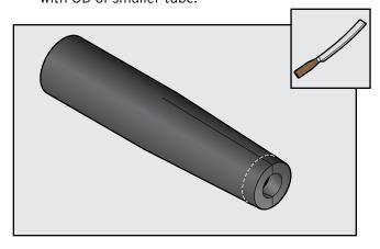
Cut end of larger ID side so length of reducer is 1/2" longer than opening to allow for 1/4" compression on each side.
