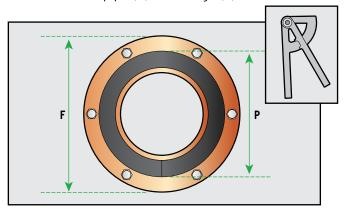
Using divider, draw inner and outer circumferences on two separate pieces of Aerocel Sheet.
