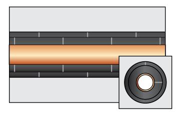
Glue butt joints under compression with Aerocel adhesive.
