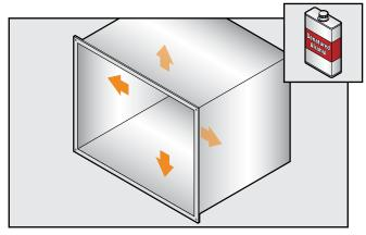
Measure duct dimensions and cut Aerocel Sheet & Roll with straight edge.
