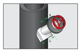
Transfer measurement of 1/2 ring circumference (1/2 c) and inner/outer strainer dimensions to Aerocel Sheet of the same thickness.
