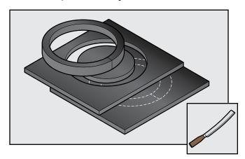
Wrap rings around pipes on both sides of flange and fully adhere to insulation inserts and bolts at flange and insulated pipes with Aerocel adhesive.
