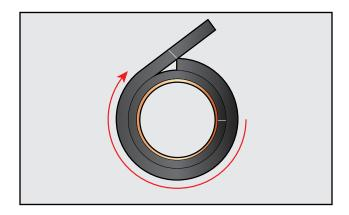
Mark and cut length of Aerocel Sheet & Roll with straight edge; add 1/4" [.64 cm] to measurement.
