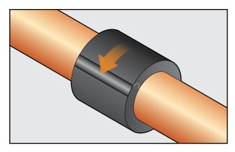
Position Aerofix so seam between the two halves is horizontal to the legs of pipe support system.
