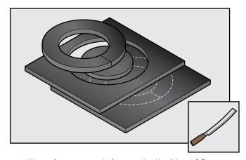
Wrap rings around pipes on both sides of flange and fully adhere to insulation inserts and bolts with Aerocel adhesive; do not glue rings to installed pipe insulation yet.
