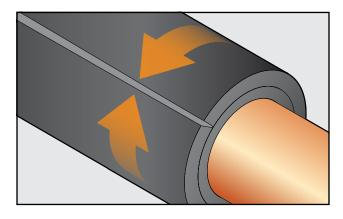
• Ensure that all longitudinal seams and butt joints are staggered; do not overlap the previous layer.
