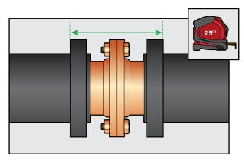
Draw with straight edge and cut flange jacket from Aerocel Sheet.
