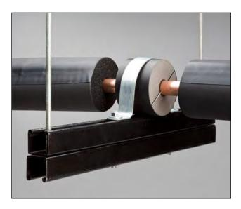
Open Aerofix fitting, remove two inside release liners, wrap around pipe, center at hanger location and press two halves together.
