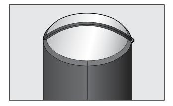
• Transfer diameter measurement to Aerocel Sheet, draw radius and then circumference.
