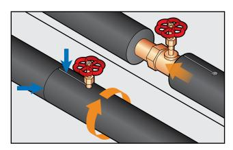
Glue valve stem, seam between valve stem, end of tube and butt joint under compression with Aerocel adhesive.
