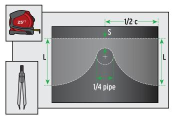
Cut strainer cover along marked lines and miter inside edge to be adhered to strainer body to ensure flush fit (do not stretch).
