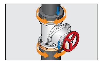
Measure circumference of rings (C) with strip of Aerocel Sheet that is the same thickness (do not stretch); add 1/4" [.64 cm] to measurement.
