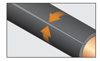
Glue butt joints under compression with Aerocel adhesive.
