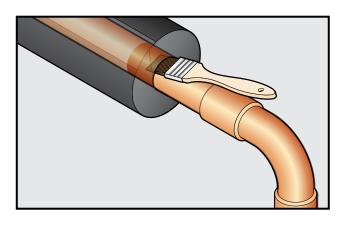
Glue adjoining tubes and fittings with Aerocel adhesive following <u>BEST PRACTICES/</u> <u>AEROCEL ADHESIVES.</u>
