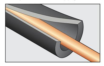
Slit flattest side of tube along 6' [1.8 m] longitudinal seam with sharp non-serrated knife; maintain knife at low angle to prevent tip from cutting inside wall of tube.
