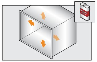
Measure duct dimensions and cut Aerocel Sheet & Roll with PSA with straight edge.
