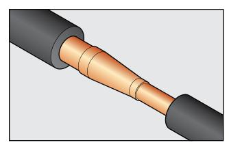
With piece of Aerocel tube the same ID as larger pipe, cut a section larger than opening between straight run tubes installed on either side of pipe transition.
