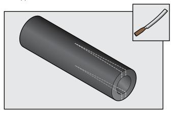
• Glue notched edges together with Aerocel adhesive
