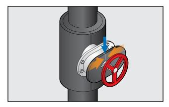
Measure circumference (C) of cover with strip of Aerocel Sheet the same thickness (do not stretch); add 1/4" [.64 cm] to measurement.
