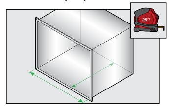
Note: Add 1/4" [.64 cm] to all measurements for compression-fitting seams (not stretched, no gaps).
