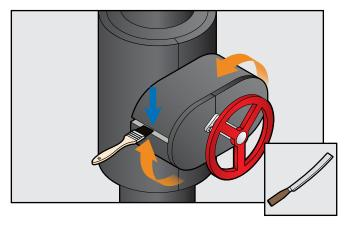
Glue edges of spindle housing jacket to valve cover body with Aerocel adhesive under compression.
