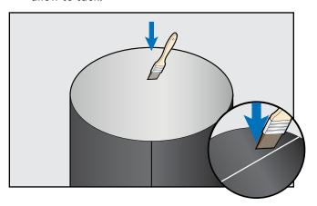
When adhesive is ready for contact, apply to dome pressing down firmly from the center to outer edges.
