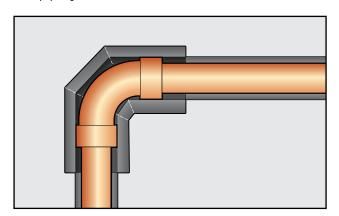
4-Piece Elbows - Welded (fitting & piping same diameter)
