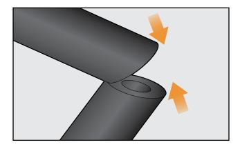
Continue until all four (4) duct flange cover components are cut.  Glue three (3) of the four (4) 45° seams with Aeroseal or Aeroseal LVOC Black to create flange cover.
