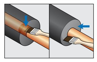
Glue longitudinal seams, butt joints and fittings with Aerocel adhesive. BEST PRACTICES/AEROCEL ADHESIVES
