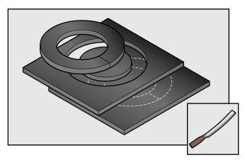
Wrap rings around pipes on both sides of flange and fully adhere to insulation inserts and bolts at flange and insulated pipes.
