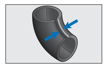
Once glued inside seam is ready for contact, wrap the fitting cover around pipe bend and apply firm pressure to ensure complete adhesion.
