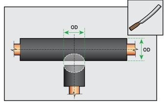
Punch hole in tube to insulate main (horizontal) pipe with sharpened pipe end of right diameter; use divider to cut hole for larger pipes.
