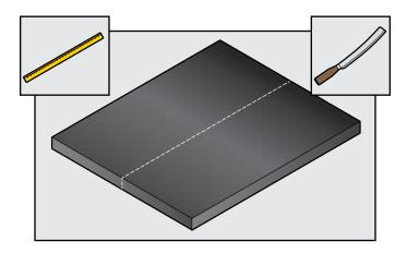
Apply Aerocel adhesive to cut edges of longitudinal seam, allow to tack up until ready for contact.
