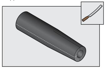
Glue reducer seam and butt joints under compression with Aerocel adhesive.
