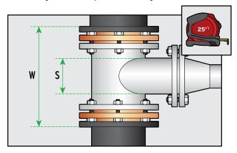
On Aerocel Sheet, mark and cut width (W), ring circumference (C) and diameter of spindle (S); mark spindle cut-out 1/8"-1/4"
