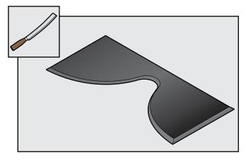
Glue strainer body cover to rings, longitudinal seam and around strainer wheel with Aerocel adhesive under compression.
