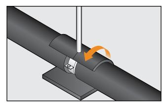
Seal all fitting cover seams and to outer surface of adjoining tubes with Aerocel adhesive to provide complete vapor seal.
