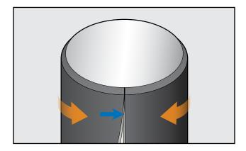
Measure the diameter of the dome using a strip of Aerocel Sheet insulation of same thickness.
