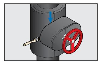
Glue edges of spindle housing jacket to face plate cover with Aerocel adhesive under compression.
