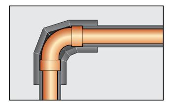
• **5-Piece Elbows - Welded** (fitting & piping same diameter)
