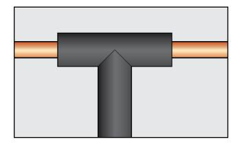
Using Aeroflex Template, cut two 45° angles to center at end of tube for branch (vertical) pipe.
