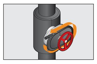
On Aerocel Sheet (same thickness), lay circumferential strip on sheet and mark into 4 equal segments.
