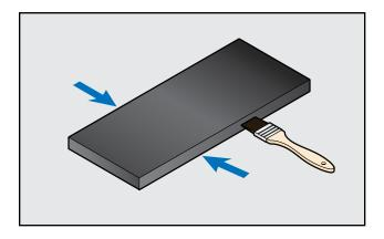
Place insulation over pipe and adhere glued longitudinal seam by pressing from the outside edges towards the middle to ensure straight edges at butt joints, full adhesion and vapor seal.
