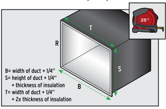
• **Note**: add 1/4" [.64 cm] to all measurements for compression-fitting seams (not stretched).
