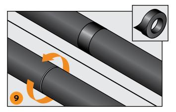
was dry to the touch prior to contact. For exterior applications, taping all glued seams with Protape is required; turn taped longitudinal seams away from direct sun exposure when possible.
